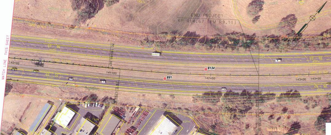
B1⊗ Approximate Naturally Occurring Asbestos & Aerially Deposited Lead Sample Location (Direct-Push)
