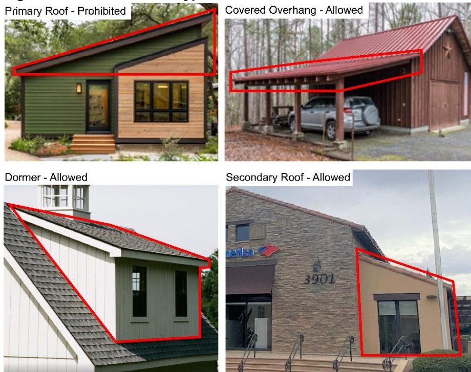
Figure 7 Shed Roof Types
