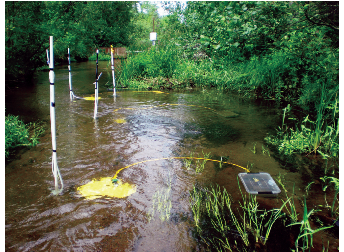
Above, seepage meters and in-stream piezometers deployed in the Shingobee River, Minnesota, to understand directions and rates of water movement between the stream and the underlying groundwater system. (Photograph by Donald O. Rosenberry, U.S. Geological Survey)
