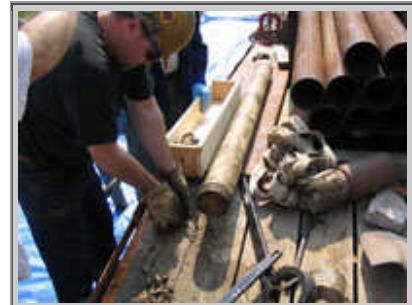
USGS scientists processing a bedrock core taken from the NAWC site (circa 2005). The core was sampled near fractures and the rock matrix was analyzed for volatile organic compounds (VOCs) -- from the Naval Air Warfare Center (NAWC) Research Site
