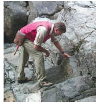
Fractures form complex paths for fluid movement in fractured-rock aquifers. Mapping rock types and fractures, where the rock is exposed, enables scientists to link fracture orientation, the interconnectivity of fractures, and fracture length with the availability of water.
