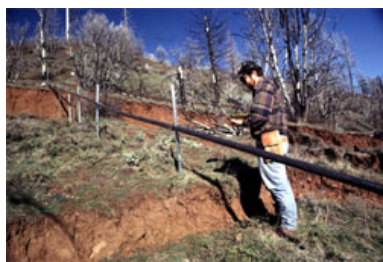
Photo 5: Measuring landslide movement using a surface extensometer. Extensometer crosses several scarps (breaks that expose the reddish soils) at the head of the landslide. USGS Photo by Richard LaHusen, USGS/CVO
