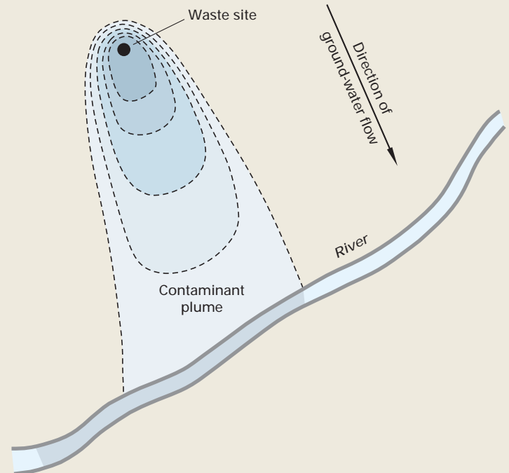
Figure M-1. The transport of contamination from a point source by ground water can cause contamination of surface water, as well as extensive contamination of ground water.
