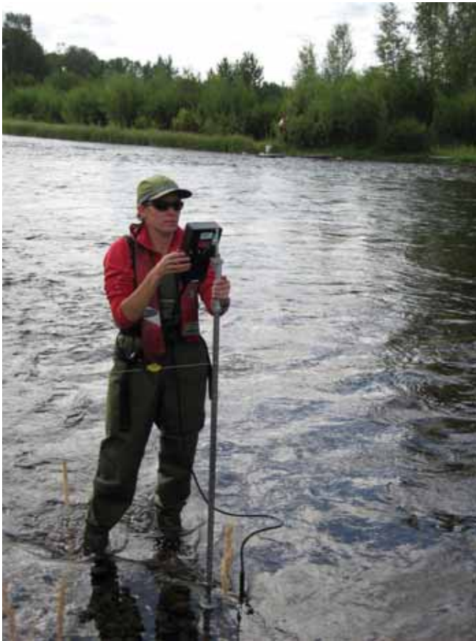
Streamflow measurement on Fish Creek, Teton County, Wyoming. (Photograph by Jerrod D. Wheeler, U.S. Geological Survey)
