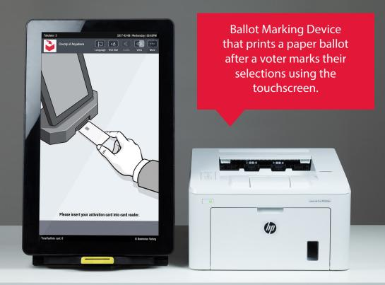
The ImageCast<sup>®</sup> X can be configured as a Ballot Marking Device (BMD), which is paired with a commercially available, compact laser printer that prints a summary of the voters selections. No votes are stored on the ImageCast<sup>®</sup> X when in the BMD configuration.
